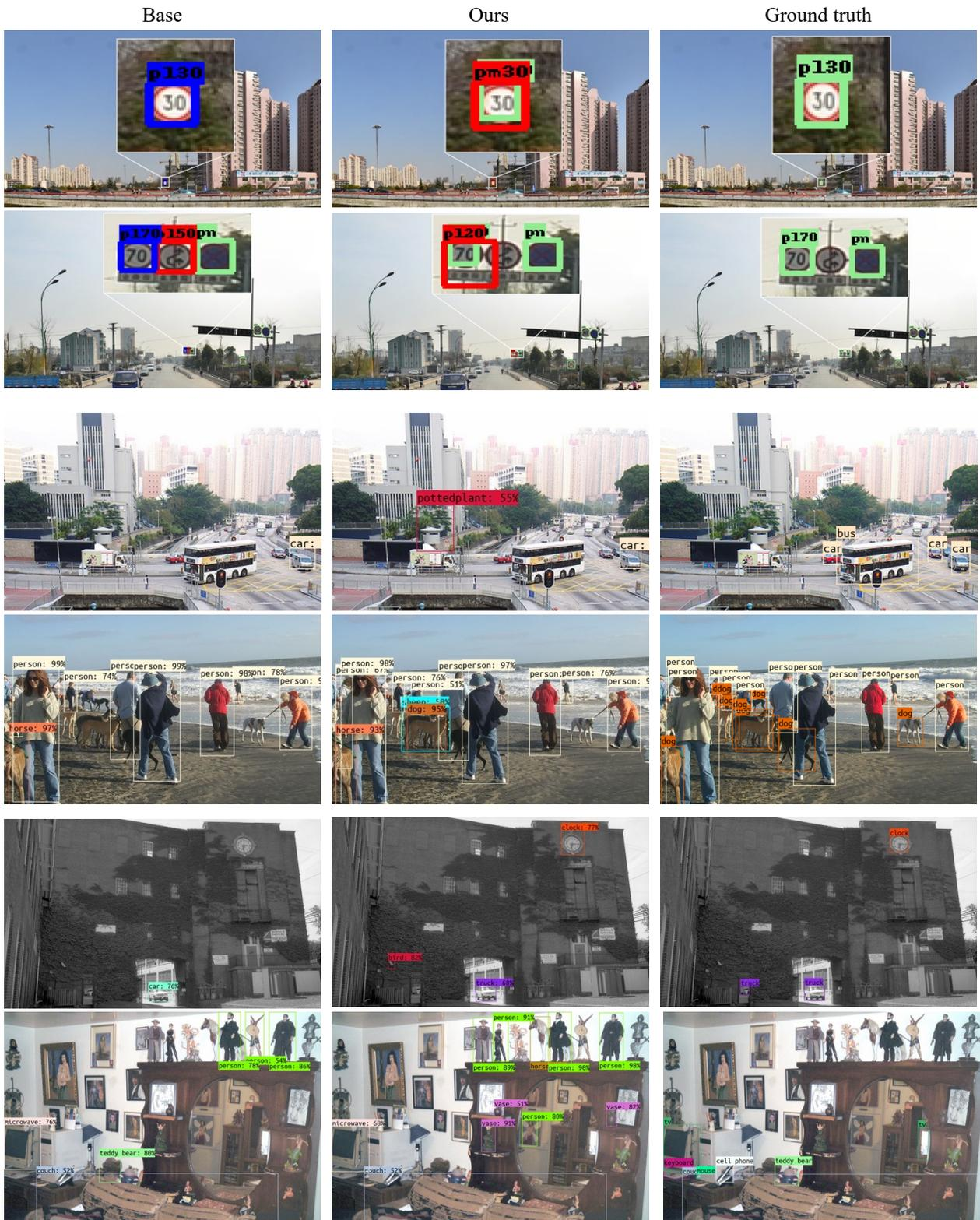
Figure 12: Failure cases on Tsinghua-Tencent 100K (row1 and 2), PASCAL VOC 2007 (row3 and 4) and MS COCO 2017 (row5 and 6) datasets. For Tsinghua-Tencent 100K, green, red and blue rectangles represent true positives, false positives and false negatives, respectively. For each row, we show the test result of the base model (left), our model (middle) and groundtruth (right). The background is cropped out of some images for better visualization.
