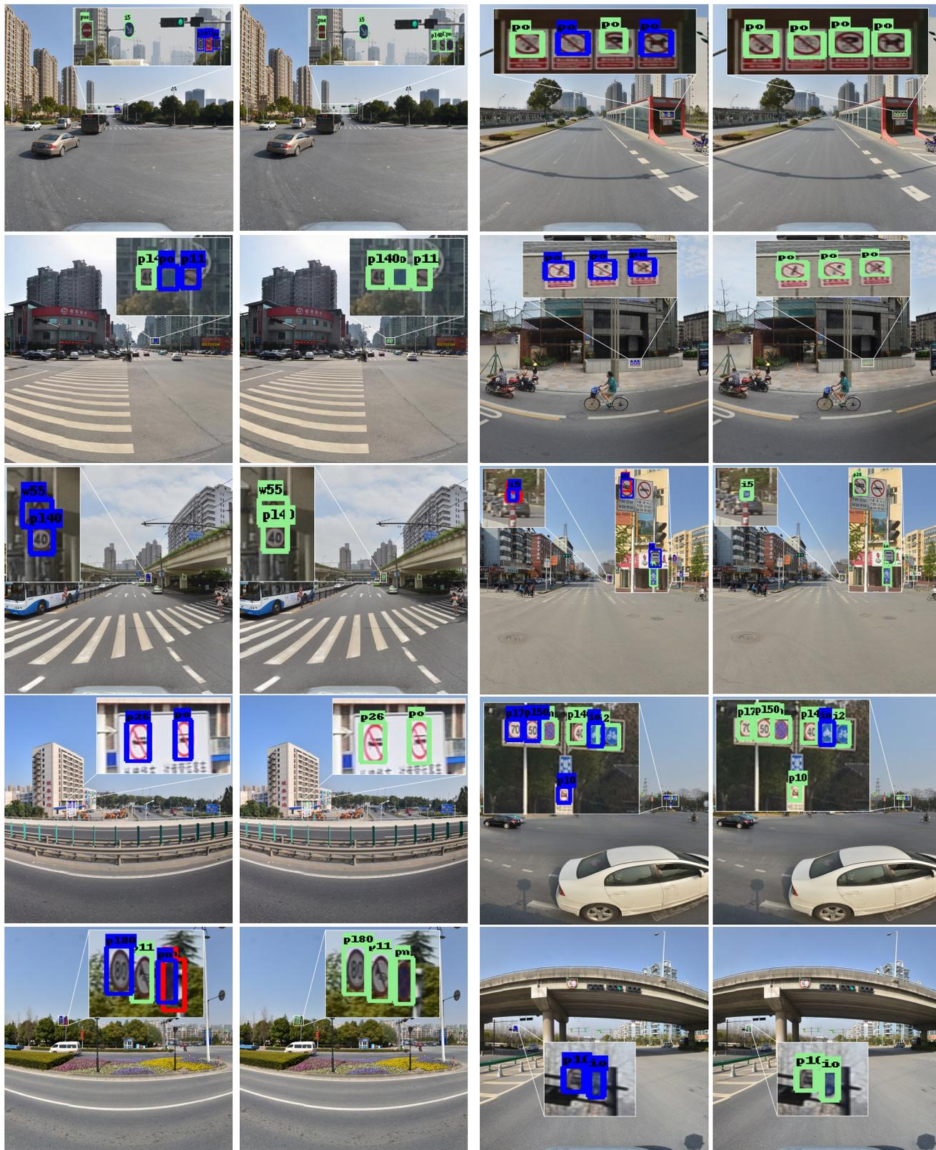
Figure 13: Detection examples on Tsinghua-Tencent 100K *test* dataset. Green, red and blue rectangles represent true positives, false positives and false negatives, respectively. Each pair indicates the results from the base model (left) and our model (right)
